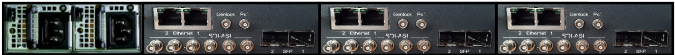
Sivac-one Frame rear panel with 3x SMP1000 MODULES integrated and redundant PSU
